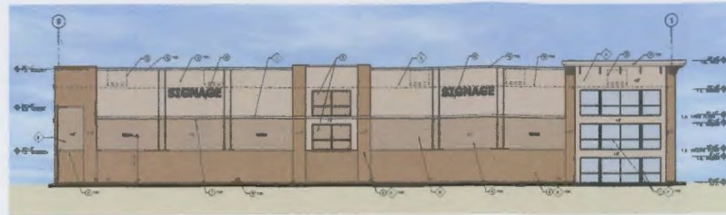
2 EAST ELEVATION - STREET SIDE SCALE: 1/8" = 1'-0"
